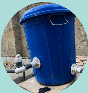
Solid filtration by sedimentation component
