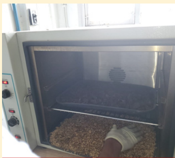
Thermal processing of dry digestates (pyrolysis)
