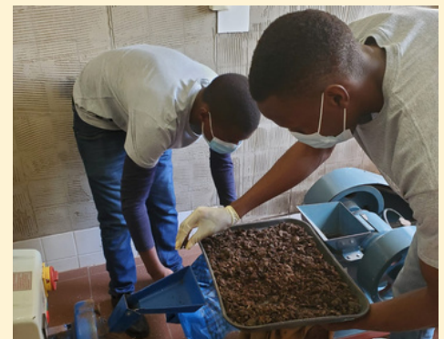
Granulation of dry digestates
